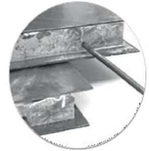
Steel-Aluminum foam-Sandwich (SAS) with integrated steel tubing
