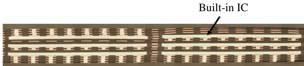
WABE Package® section structure
