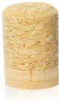
**Champagne corkstoppers** are produced from a body of agglomerated cork to which one or two discs of selected natural cork are glued to one of the ends. These stoppers are designed for champagne or sparkling wines and have larger diameters than regular wine corks for retaining the high internal pressures in these wines. Champagne corkstoppers are available in different classes depending on the visual quality of the outer disc and in different sizes from which the most common ones available are:
