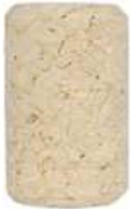
**Agglomerated corkstoppers** are produced entirely from cork granules obtained from granulation of by-products resulting from the production of natural stoppers. They can be produced by individual moulding or by an extrusion process and the cork granules are binded together by an agglutinating substance approved for contact with foods. These corks are usually used for sealing bottles with wines of rapid consumption. These corks may have diverse sizes depending on its intended use.
