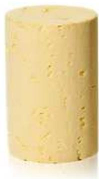
**Colmated corkstoppers** are natural corkstoppers with surface pores and irregularities filled with selected cork powder resulting from the natural stoppers production process. A food-grade glue based on natural resin and natural rubber is used for adhesion of the powder. These stoppers are of quite homogenous appearance and provide an alternative to natural corkstoppers for sealing rapid consumption wines.
